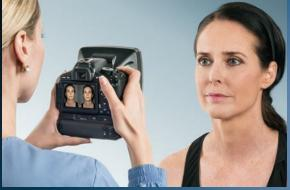
Integrated flash and converging ranging lights for fast, reproducible imaging every time.
